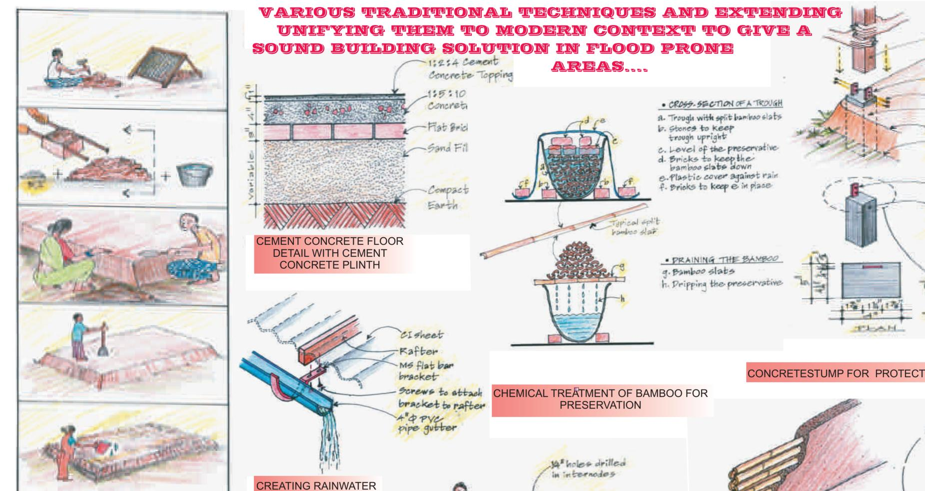
CONCRETESTUMP FOR PROTECTING LOWER END OF BAMBOO POST
